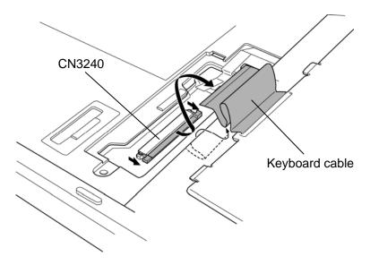
Figure 4-17 Removing the keyboard
